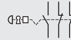
Mushroom head Emergency stop Turn to release, trigger action key release N/O + 2 N/C contacts
